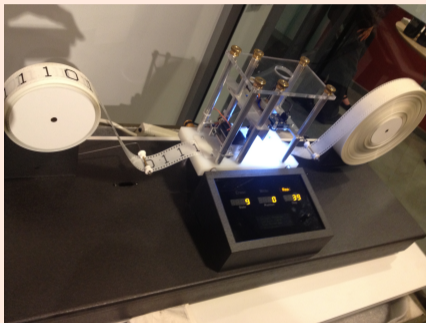
Figure 16: Real-life implementation of a Turing machine (Source: wikimedia.org)
